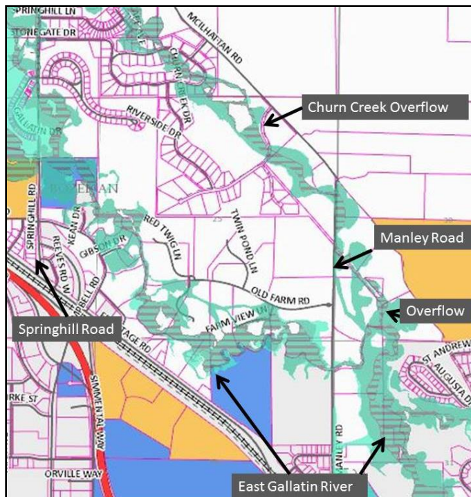
Figure 47. East Gallatin River floodplain mapping (green) showing overflow from point upstream of Manley Road.
