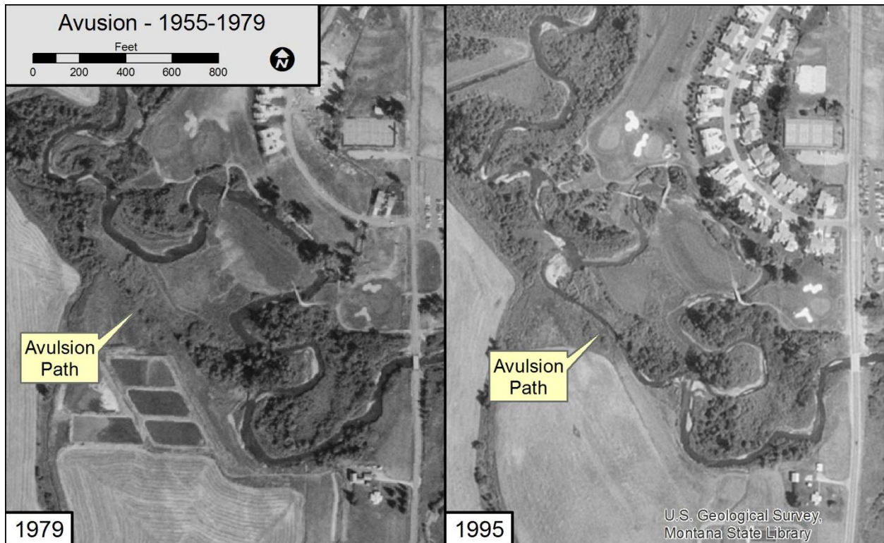
Figure 52. East Gallatin River at Bozeman Water Treatment Plant showing avulsion between 1979 (left) and 1995 (right).
